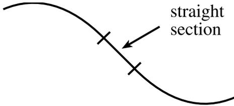
The crossover between two turnouts forms an "S" curve, but this is unavoidable and will be allowed, even between mainline tracks.
